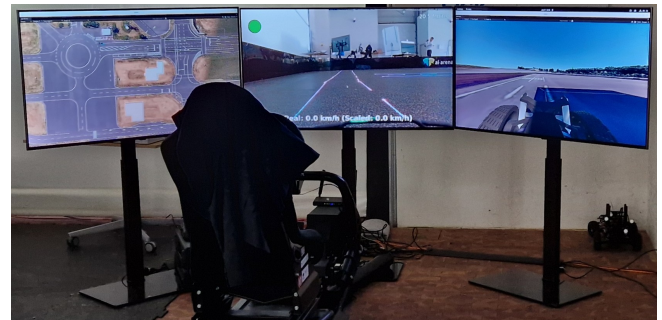
(c) Operator workplace at the scaled test field set up for remote driving with co-simulation to the side.
