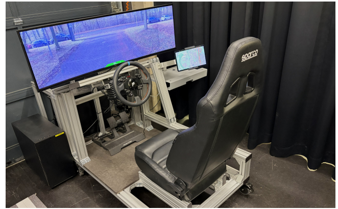
(a) Portable operator workplace: an ultra-widescreen monitor and a tablet to assess the scene, a steering wheel and pedals remotely control the vehicle.
