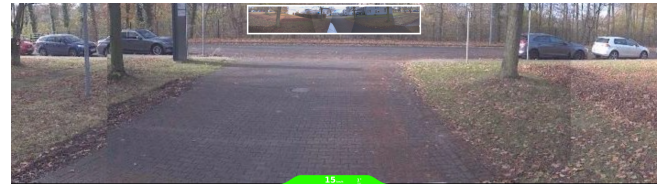
(b) Remote driving Graphical User Interface (GUI) of operator workplace showing a stitched frontal (and rear/side) multi-camera view: speed, steering wheel angle, and system engagement status are displayed.
